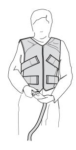
Attach the end of the Connector Hose to the Connector Port on the Vest by firmly inserting the two pieces straight into each other. There should be an audible "click". The Connector Hose should be oriented so that the disconnect button is facing away from your body.
